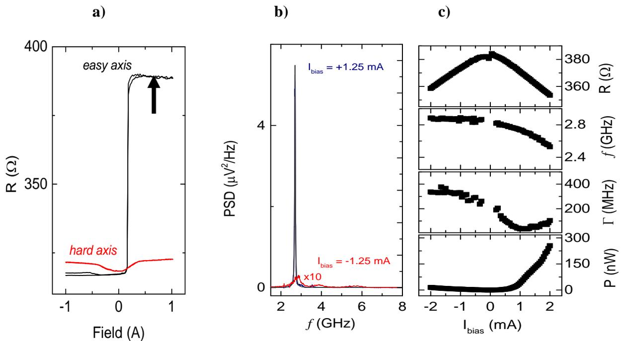
**Figure2:** a) Transport measurement (two contact measurement) in easy and hard axis. The arrow indicating the RF measurement point b) Microwave emission spectra measured in positive bias currents (Black spectrum) and negative bias currents (Red Spectrum). c) Shows the results, in terms of power emissions, linewidth, frequency tunability and resistance.
