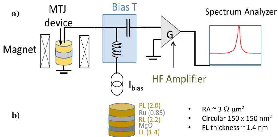
**Figure1:** a) Illustration of radio frequency (RF) measurement setup. b) The measured MTJ stack and nanopillar dimension.
